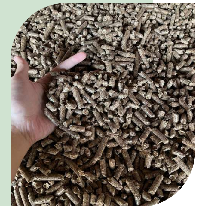
Above: Wood pellets sourced by Nova Energy for the coal-to-wood pellet conversion trial.
